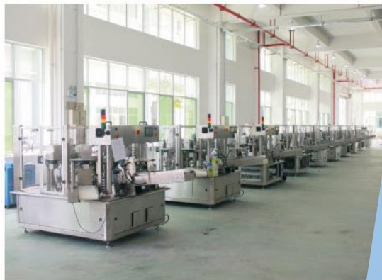
給袋機車間 Doypack machine workshop
