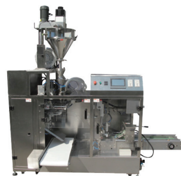
AP-1BT with screw auger for powder
